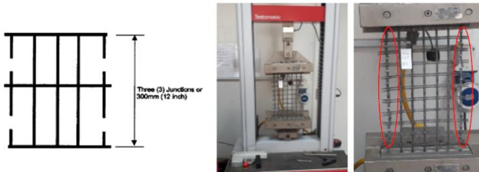
Figure (2): Specimen configuration; Multi-Rib tensile method -ASTM D6637
