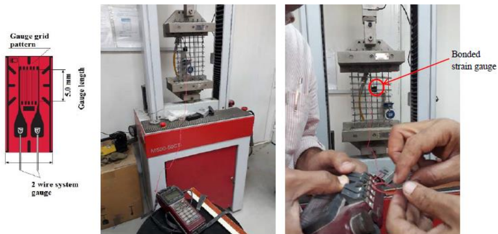
Figure (2): Test setup for Calibration Factor between local to global strain using CSR tensile test
