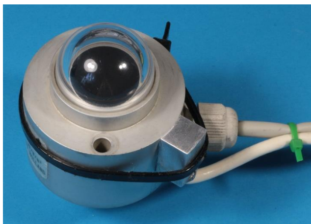
Figure 5. A fixed Pyranometer
