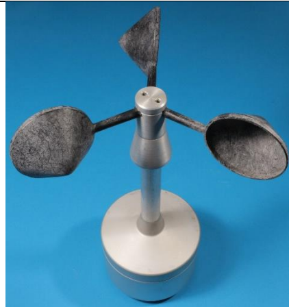
Figure 6. A fixed wind velocity measuring device (anemometer)
