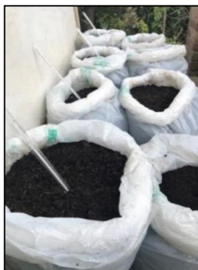
Figure 1. Pilot Scale Composting Systems with thermometers (static piles) (Source: The authors)
